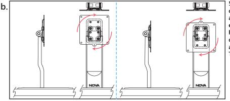
5b. VESA plates can be detached and rotated to ensure a monitor height clearance of 1 1/2" to 2" above the closed Trolley™ door.
