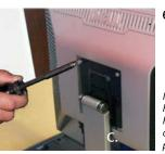
6c. Attach monitor to VESA plate using the four removed monitor screws.
