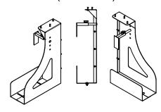
Mounts to underside of work surface. Fits CPUs up to 18" high.
